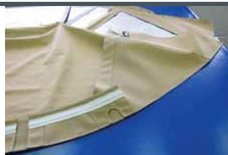
5 In this step we are joining the aft pocket and the wings in one seam. This is the area of concern for some fabricators. Notice the stacking order of the pieces. Also notice that the pocket extends inside the wing by about 6 inches on each side. This particular dodger has straps instead of bars aft so we have included cutouts just inside the wings to accommodate them.
