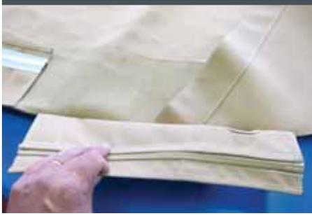
6 Here is a peak under the lid. Notice that the wing is stapled down first with the pocket on top. Notice that our aft pocket is in three sections with a gap between them. This is so our aft welded handle can pass through and be zipped onto the aft frame.
