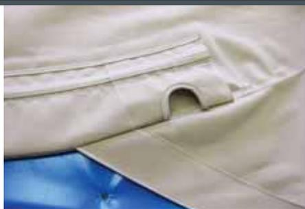
10 We have flipped the dodger to the backside and turned the pocket to the inside. The aft pocket has been stitched down through the top football panel and leather chafe below it. No need to ease off the ends of the aft pocket because it extends far enough down the side of the dodger not to be a problem. Notice that the wings extend out from the middle of the seam between the top football panel and the aft pocket.
