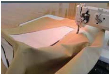
3 We are topstitching the seam between the top football panel and the forward panel assembly. The seam contains the forward pocket. Be sure when topstitching that the forward pocket faces out under the forward windows.
