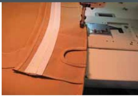
7 In this photo we are stitching a 1/2-inch hem along the entire aft edge. We back tack in areas of high stress, such as the bottom edge of the strap cutout that has to bear all the down pressure of the strap.
