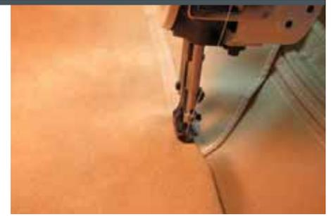
8 We are topstitching the entire aft seam of the dodger. In the photo we are about to topstitch over the interconnection between the pocket and the wing. Be sure that the aft pocket in this step faces out under the wing.
