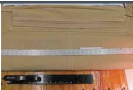
4 After topstitching, flip the assembly over and stitch down the forward pocket. It is important to ease off the ends of the forward pocket by  $\frac{1}{4}$  inch—only the center needs to be tight. We have mentioned this before in past articles, but it is so important to do this that it warrants repeating: If you were to stitch this forward pocket down flat along the straight line in the photo you would have diagonal ripples in your top panel.
