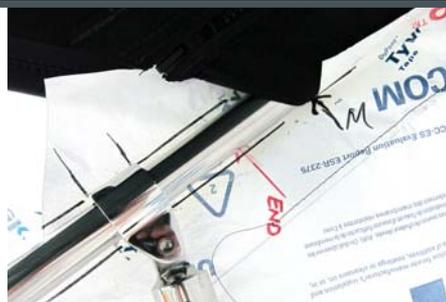
**10** This is an inside view of our top pattern in the corner of the bimini. Notice the black arrow match mark at the corner of bimini pocket. The bimini pocket is 1½ inches up from side of bimini. We overlap all bimini corners by this amount to prevent gaps and leaks. The natural intersection is just to the right of match mark in the photo at the same level. The enclosure panel extends up to the bottom of the bimini pocket to hide the zipper.
