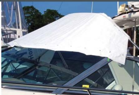
2 Here we are patterning the forward windshield after removing the pattern from the top and sides. Be sure to mark and label the same match marks on this piece. When marking the forward bow on both pattern pieces, be sure the lines are close to identical along the forward edge.
