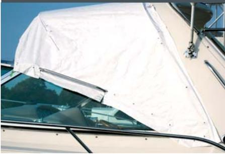
1 In this photo we are patterning the sides and top together as part of our one-step patterning process. We have put match marks on the frame at the bimini corners and at a snap on the windshield directly below the corners. These match marks are transferred to both pattern pieces and enable us to align and tape the pieces together back at the shop. We use double-sided tape to hold the patterns to the frame, arch and windshield to speed the process.
