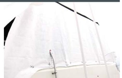
**11** The side zips are sewn onto a straight line at the top of the side pattern. Correct the top zip angle with darts using hash marks between the fasteners, as in the photo.
