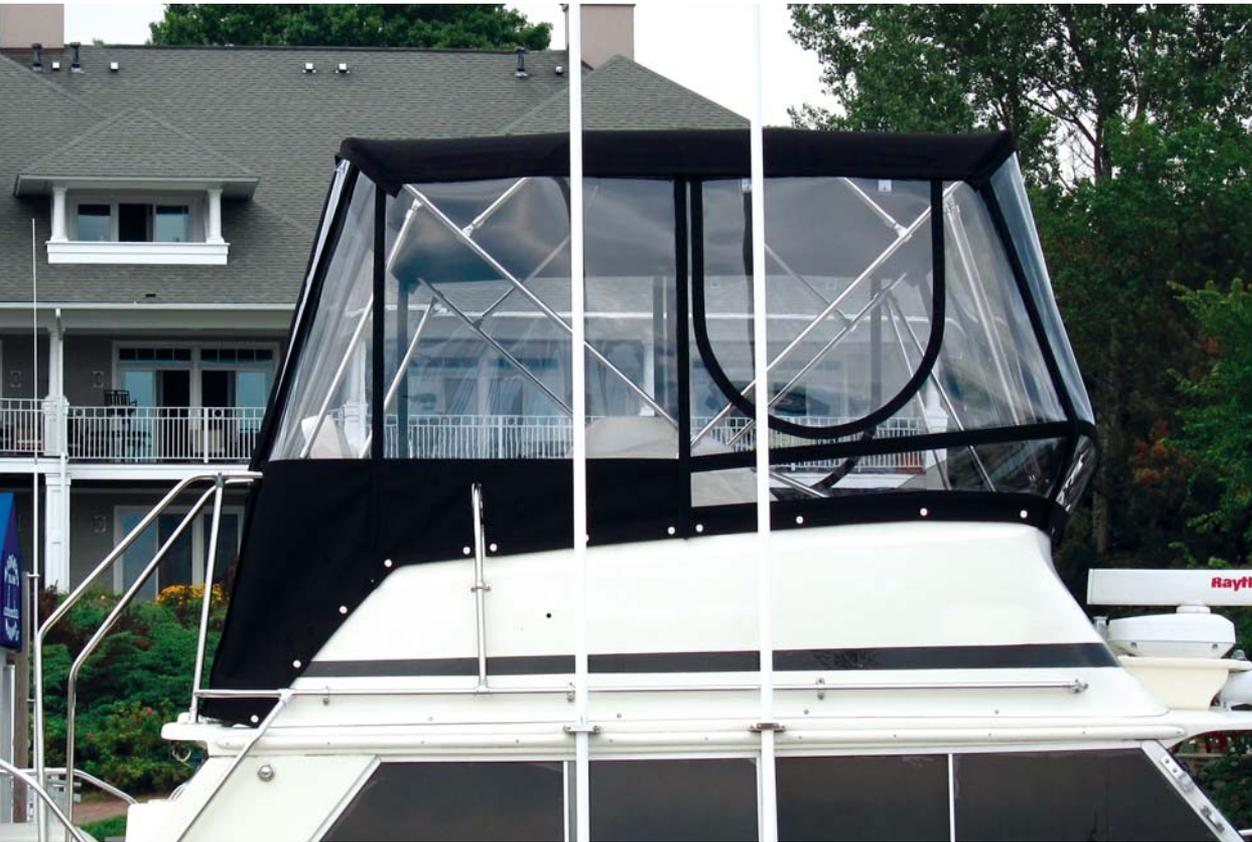
Our completed bimini enclosure. The vertical division at the corners originates at the Natural Intersection under the visors.
