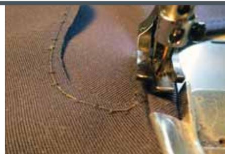
6 We are at the corner in this photo. If we were to go any further, the needle would have stitched over the fold. Always pay attention to the needle position to avoid doing this. Staple pullers, inverted as a finger extension, can be a useful tool for getting the fabric to where it needs to be relative to the needle.
