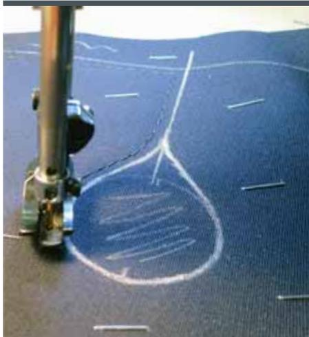
1 We always have two layers of fabric wherever there is a cut out. In the photo, we have marked the fabric from our pattern and stapled the plies together. We are stay-stitching along the bottom of the panel and up and around the cutout. With sharp scissors, cut on the white lines, and heat the edges with a hot knife.
