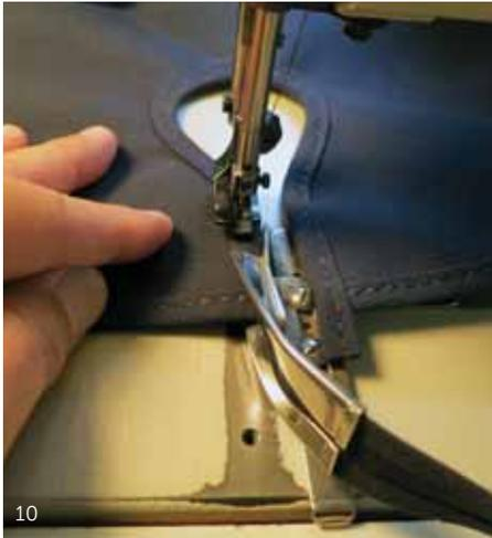
7 – 10 This fold-and-stitch process is repeated all the way around the curve 2 to 3 stitches at a time. A DC servo motor can be a real plus here for low speed control while binding curves.
