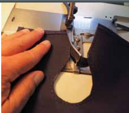
2 Here we are positioning our binder with the cutout in position to be bound. Notice we have bound the bottom edge first. This way mistakes going around the cutout can be removed easily with the small blade of a jackknife under the edge. Hold the blade flat on the fabric and insert the tip under the edge of the binding to be removed and draw the blade along the length of the binding, cutting the thread. It is best to use a semi-sharp blade: It makes binding removal fast and painless.
