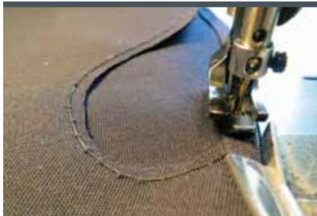
4 We are approaching the first inside curve. Our fabric is folded hard left, back on itself. The needle is advanced as far as it can go without stitching over the fold.
