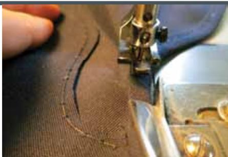
5 With the needle down, we pull the fabric fold to the left of us up and to the left. This pull of the fabric gains us about 2 to 3 stitches before we are forced to another corner.
