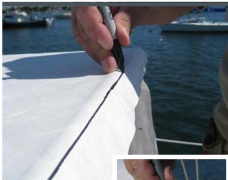
4 We have stuck our one-piece top and side-pattern blank onto the sticky tape between the frames. Start at the center line and alternate, so the pattern lays flat down each side. Secure with fasteners at the bottom of each side. Draw a line on the aft bow holding a consistent 45-degree angle to the top of the bow along the entire aft edge.
