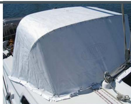
6 This is the forward view of the paper dodger. Notice the hash marks drawn along the forward bow seam. Also, notice the hash marks where the two patterns meet. These hash marks are important for proper alignment during pattern development and sewing the forward seam.
