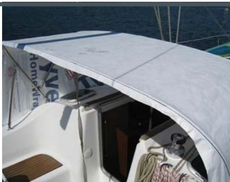
5 This is a rear view of the paper dodger with the aft bow line drawn at the correct angle.
