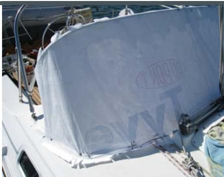
2 At the bottom, we screw our fasteners through the pattern to hold it in place. A piece of duct tape on the backside of the pattern at the fastener location reinforces it.
