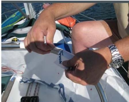
1 At the top of the forward pattern blank, we trim our pattern close, make a couple of slits and tape it to the frame.
