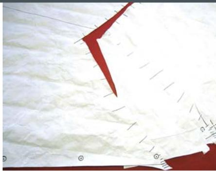
**8** We have cleaned up the bottom edges of the pattern below the fasteners and drawn our top-panel and side-curtain dividing line on the pattern. The two pattern pieces are in position to have the corner hash marks matched and joined into one with tape.
