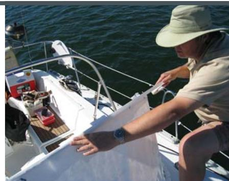
3 Next we apply a strip of 3/4-inch double-sided sticky tape on top of the forward pattern from edge to edge.
