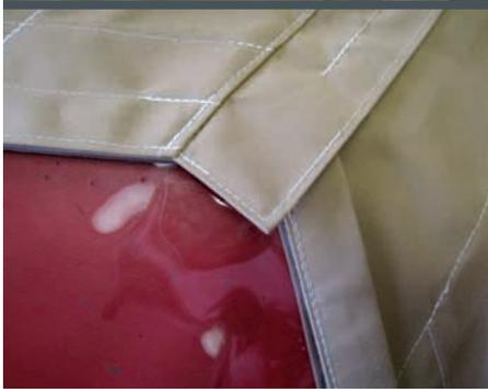
5 This is the outside of a bimini corner with a fabric angle back on the aft end, instead of a glass enclosure. Note that the vertical division extends down from the visor and not down from the pocket area of the bimini.
