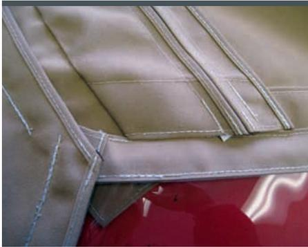
6 The inside view of the same bimini corner. Note that with the 1½-inch overlap, the width of a #10 zip, there can be no leakage on these corners.
