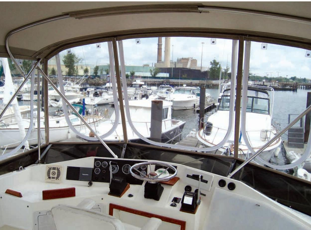
A finished bimini enclosure from the inside. Note the clean look with no zippers, the "smile" zippers showing and the "no gap" corners. This is just one way of many to fabricate enclosures that produce quality results.
